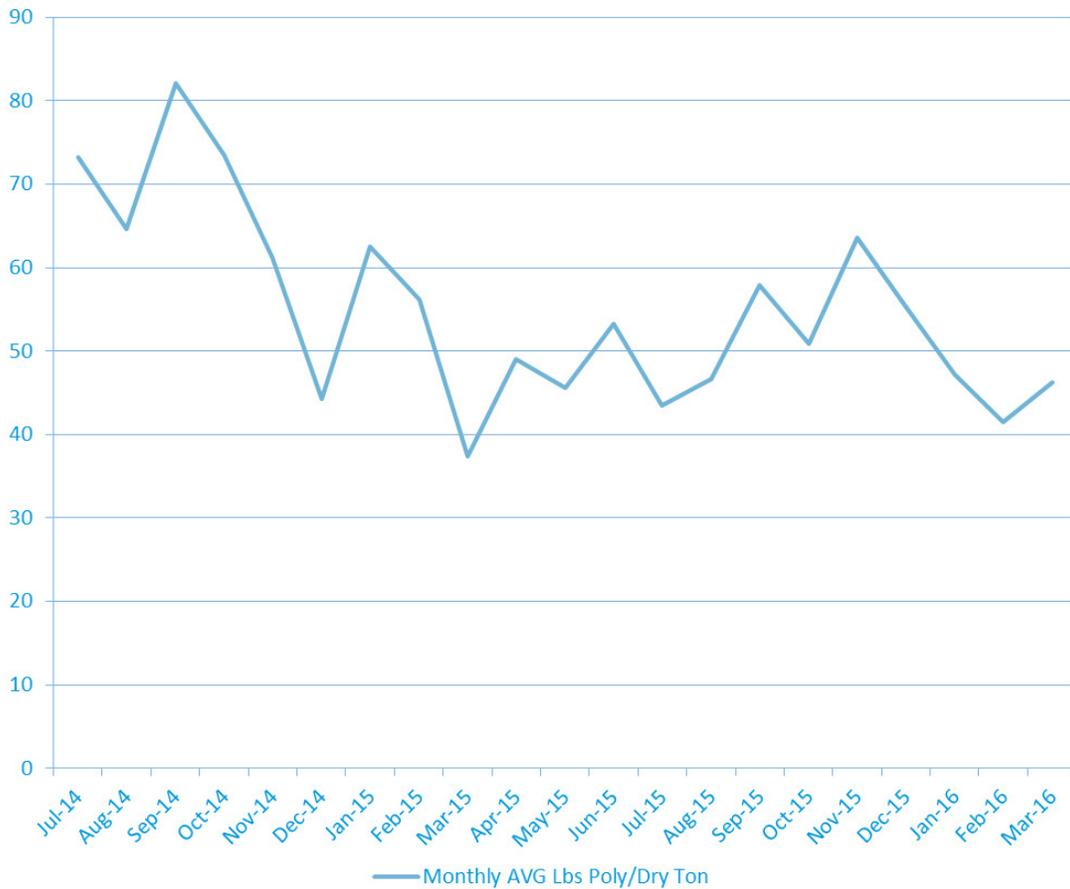
Figure 3: RTC-SD helped BGMU reduce polymer feed by 58%
